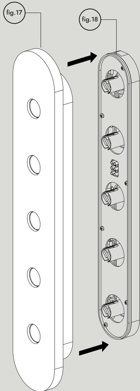
Gently install cover assembly (fig.17). Line up all five holes and mate cover assembly with main body. Take great care not to damage the lamp holders. You will feel slight resistance due to the groove gasket (fig.18), this is normal. Inner gasket (fig.16) will compress against outer edge of the main body.
