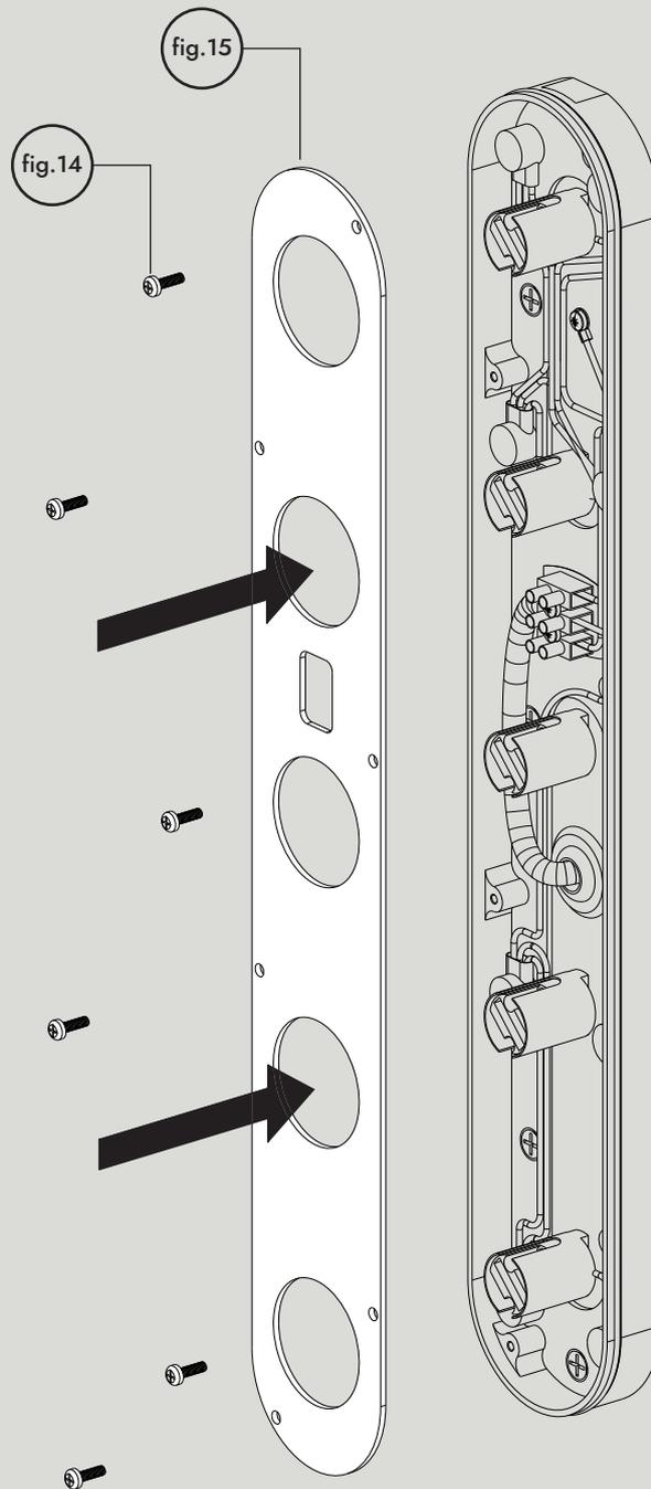
Fit cable cover (fig.15) with 6X screws (fig.14). Ensure that no cables are trapped or loose.
