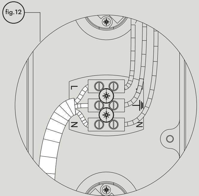
Connect the mains cable to the terminal block (fig.12). L = Brown, N = Blue
