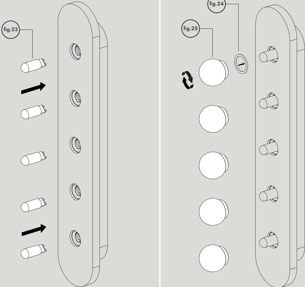
Install 5X G9 LED capsule Max 4W (fig.23) not supplied. Ensure capsule is firmly pushed in. Before screwing on glass shade (fig.25), ensure that 1X glass gasket (fig.24) is located in its place. Please take great care when handling the glass shade. Screw glass shade gently so its firmly secured. Do not over screw as this can cause the glass to break.
