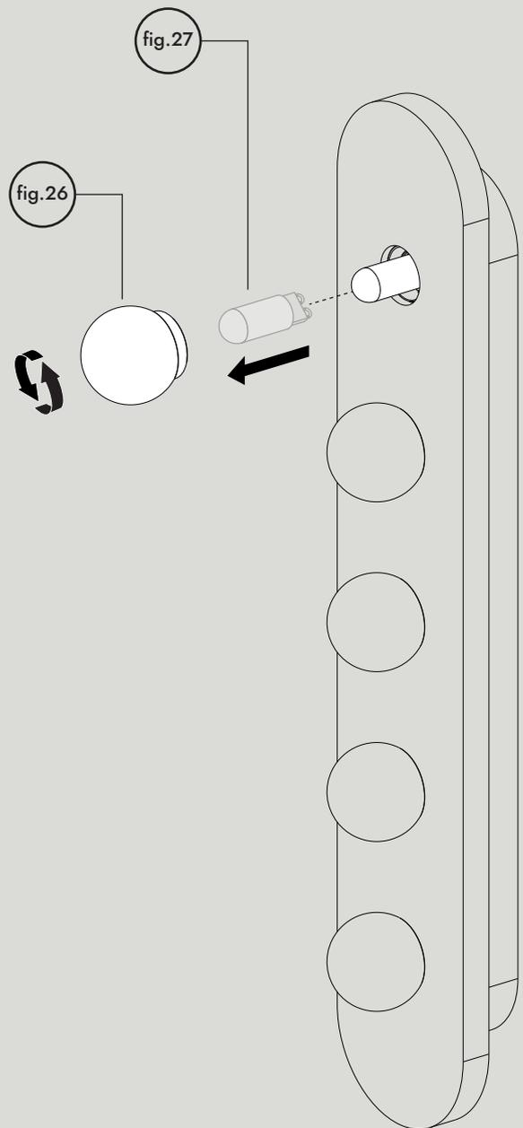
To replace LED capsule. Gently unscrew glass shade (fig.26). Hold the LED capsule (fig.27) firmly and pull in a parallel motion from the lamp holder. Do not twist as this could damage the lamp holder. To fit LED, firmly push LED into lamp holder. Ensure secure fit.
