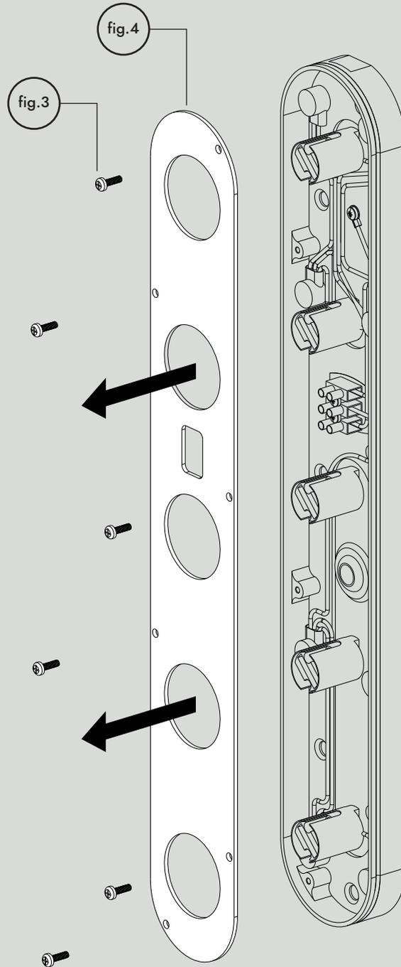
Unscrew X6 cover screws (fig.3) and remove cable cover (fig.4).
