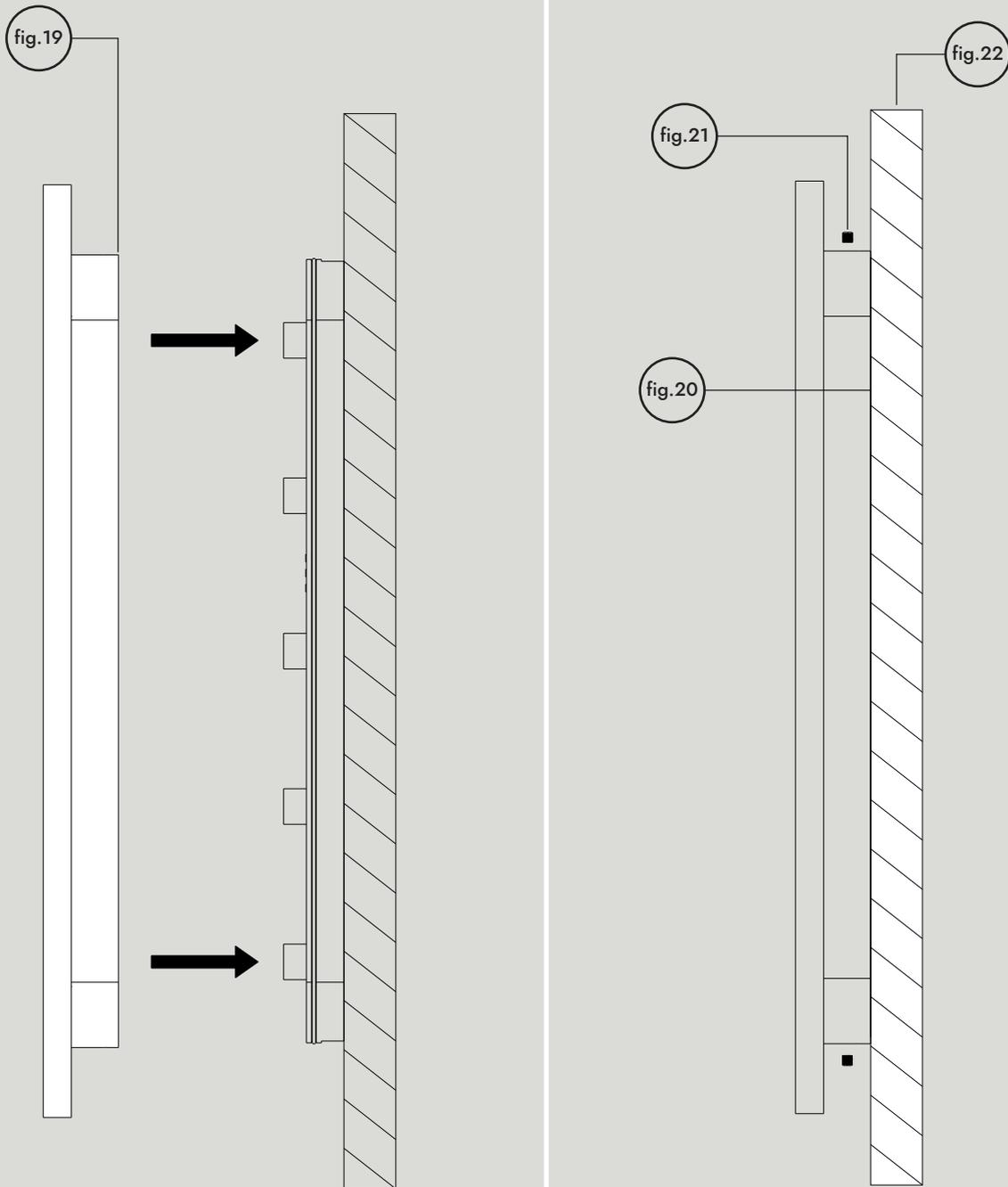
Install the cover assembly (fig.19). Ensure edge of cover (fig.20) is flush against the surface (fig.22). To achieve this gently push the cover until the edge is touching the surface (fig.22). Whilst holding the cover against the surface secure with 2X set screws (fig.21).
