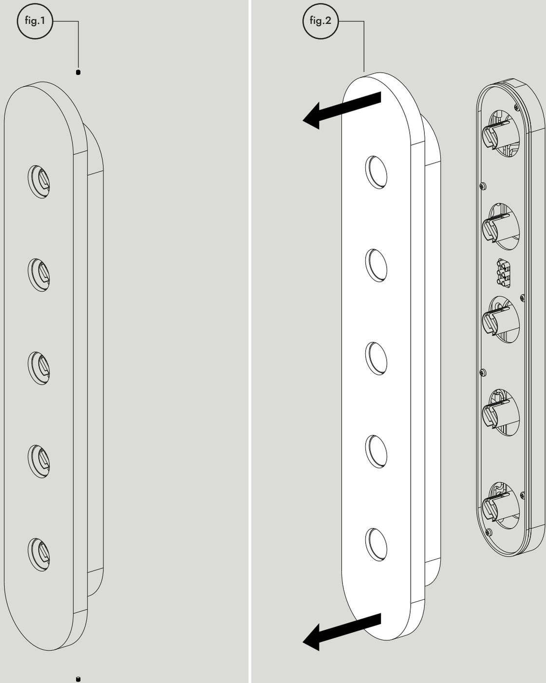
Loosen both upper and lower set-screws (fig.1). Gently remove cover assembly (fig.2), taking great care not to damage the lamp holders.
