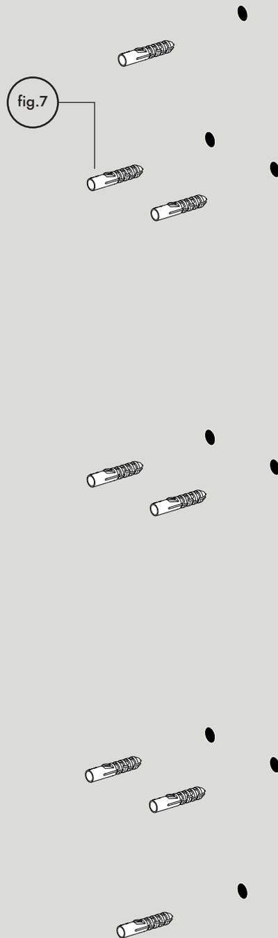
Ensure wall is flat and free from imperfections. Mark out mounting holes. Pay attention to position of cable entry to ensure correct final positioning of product. Drill holes for appropriate wall plug fixings, suitable for the fabric of the wall and fit wall plugs (fig.7) not supplied.
