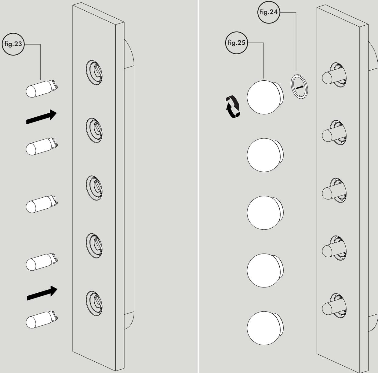
Install 5X G9 LED capsule Max 4W (fig.23) not supplied. Ensure capsule is firmly pushed in. Before screwing on glass shade (fig.25), ensure that 1X glass gasket (fig.24) is located in its place. Please take great care when handling the glass shade. Screw glass shade gently so its firmly secured. Do not over screw as this can cause the glass to break.
