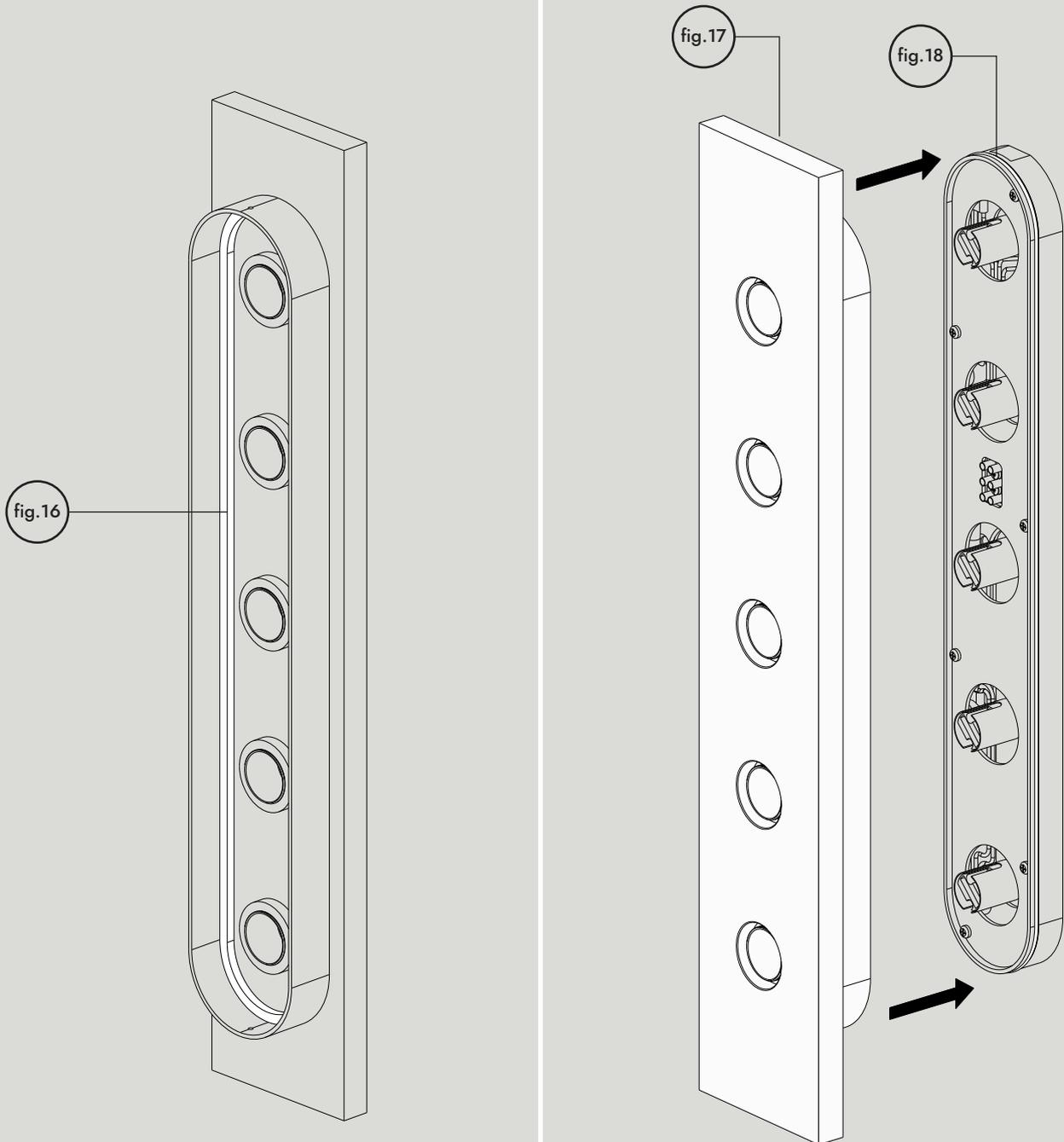
Gently install cover assembly (fig.17). Line up all five holes and mate cover assembly with main body. Take great care not to damage the lamp holders. You will feel slight resistance due to the groove gasket (fig.18), this is normal. Inner gasket (fig.16) will compress against outer edge of the main body.
