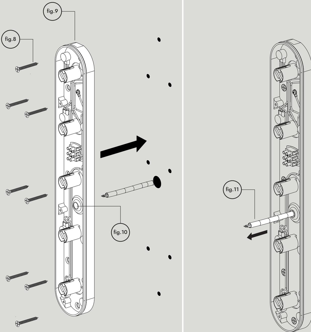
Mains cable from surface (fig.11) must be in line with cable entry on the body (fig.10). Offer cable from surface through the body. Fix body (fig.9) to surface using 6X screws supplied (fig.8). Ensure wall gasket is fully compressed on surface.
