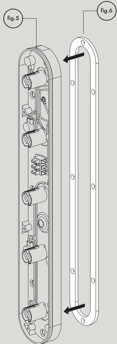
Fit gasket (fig.5) into groove on the body. Gently stretch gasket until fit is achieved. Ensure wall gasket (fig.6) is positioned within its allocated space at the back of the product.
