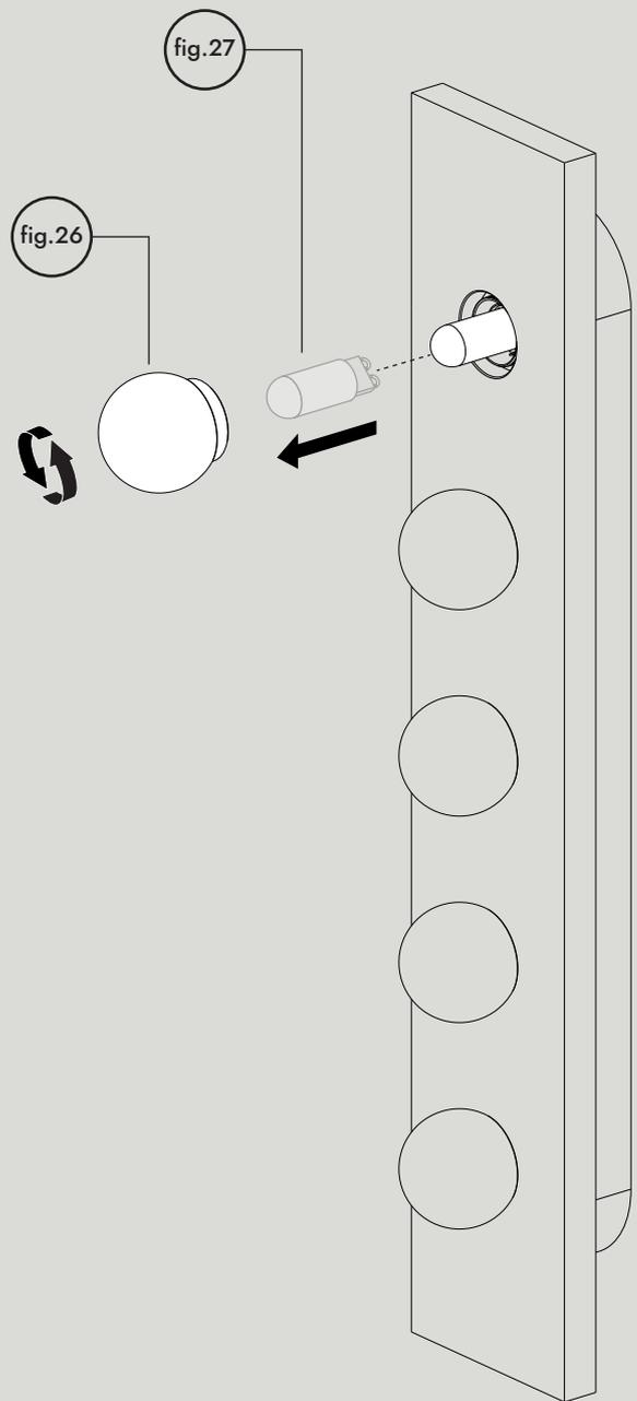
To replace LED capsule. Gently unscrew glass shade (fig.26). Hold the LED capsule (fig.27) firmly and pull in a parallel motion from the lamp holder. Do not twist as this could damage the lamp holder. To fit LED, firmly push LED into lamp holder. Ensure secure fit.
